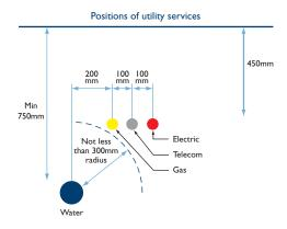
A trench shall provide no less than 750mm and no more than 1,350mm of cover to the water pipe.
