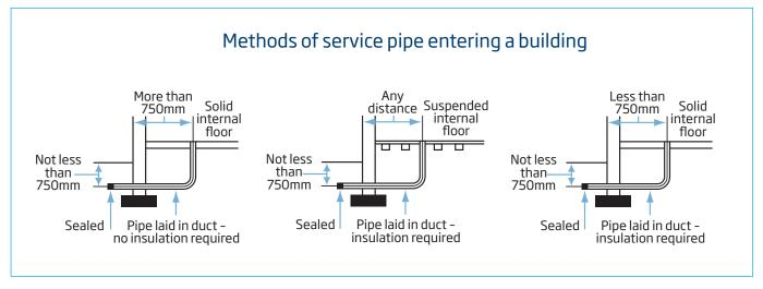
Where pipes enter the building, they must be passed through a continuous duct sized so that the service pipe can be readily removed and replaced.
